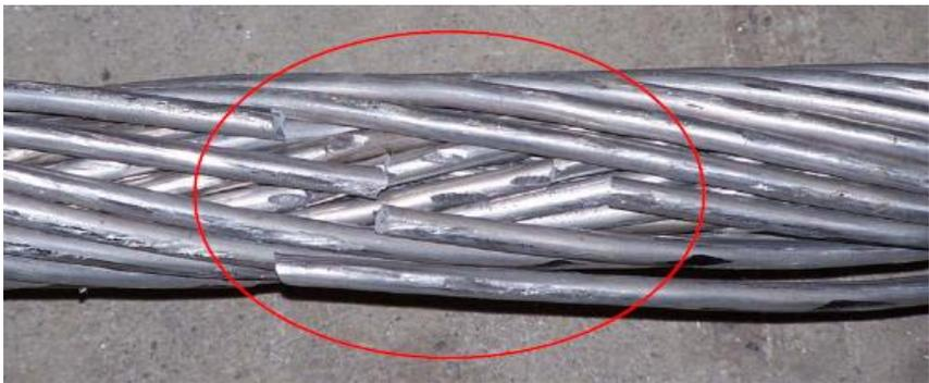
Figure 42 - Strand fretting and fatigue failure of round stranded ACSS Conductor
