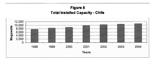
Figure 8 presents the increase in capacity for Chile, whose electricity markets were restructured in 1986. Electricity capacity in 1998 was 7544 MW, rising to 10,737 MW in 2004, an increase of 42 percent.
