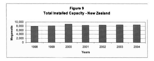
Figure 9 presents the increase in electricity capacity for New Zealand from 1998 to 2004. Similar to Australia, New Zealand's electricity markets were restructured in the late 1990s. Electricity generation capacity in New Zealand grew from 7,899 MWs in 1998 to 8,642 MWs in 2004. This represents an increase of 9.4 percent. Given New Zealand's relatively slow economic growth, this again shows that restructured electricity markets have robust incentives to induce entry into electricity generation.
