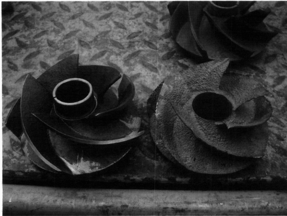
Elmwood 66 Distribution Pump - Comparison of old bronze impellers and new ductile iron impeller
