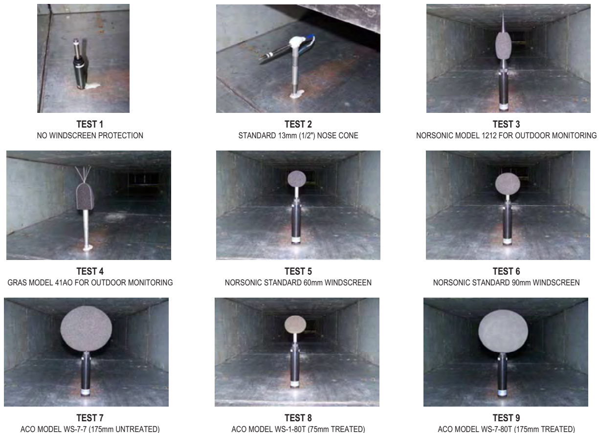
Fig. 2—Photographs of nine microphone test configurations.
