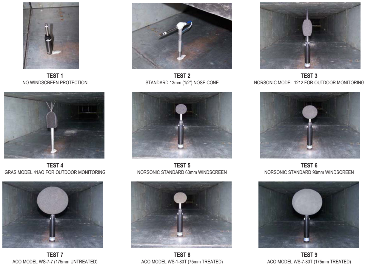
Fig. 2—Photographs of nine microphone test configurations.
