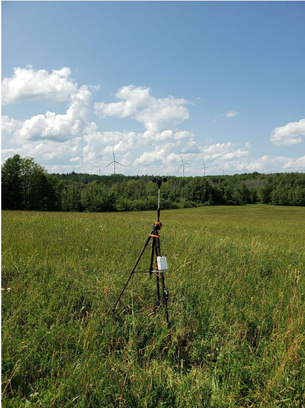
Figure 1-3 Location 1 - Meteorological Tower
