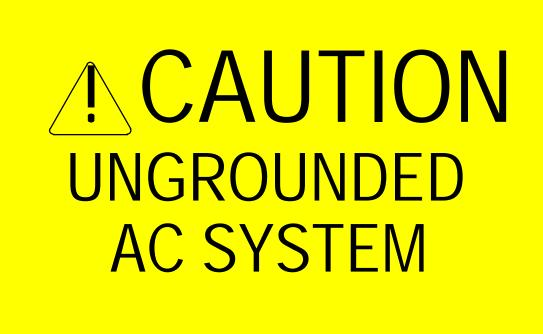
TO BE POSTED AT EACH MEDIUM VOLTAGE TRANSFORMER & INVERTER ON THE LOW VOLTAGE SIDE
