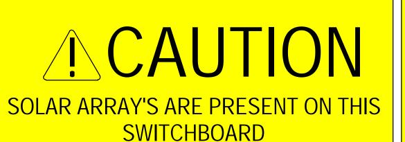
TO BE POSTED BY THE SWITCHGEAR PER NEC 705.10
