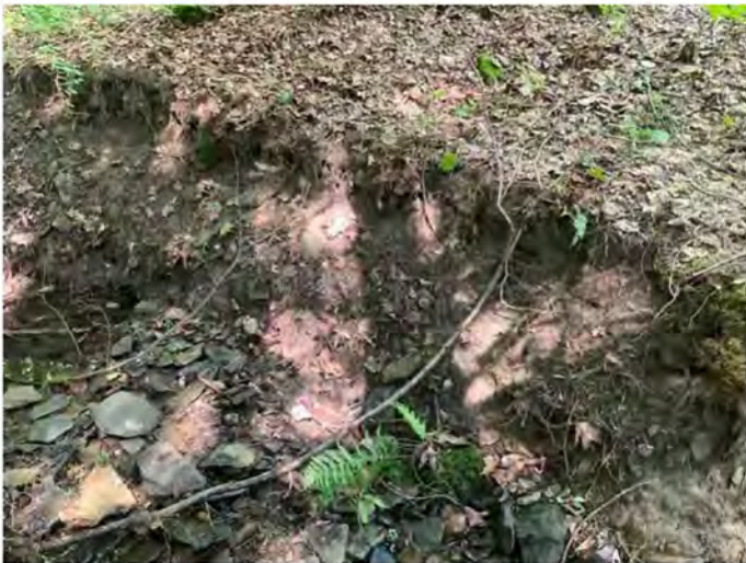
Exposed roots within intact soil layer, break in slope, change in particle size distribution
