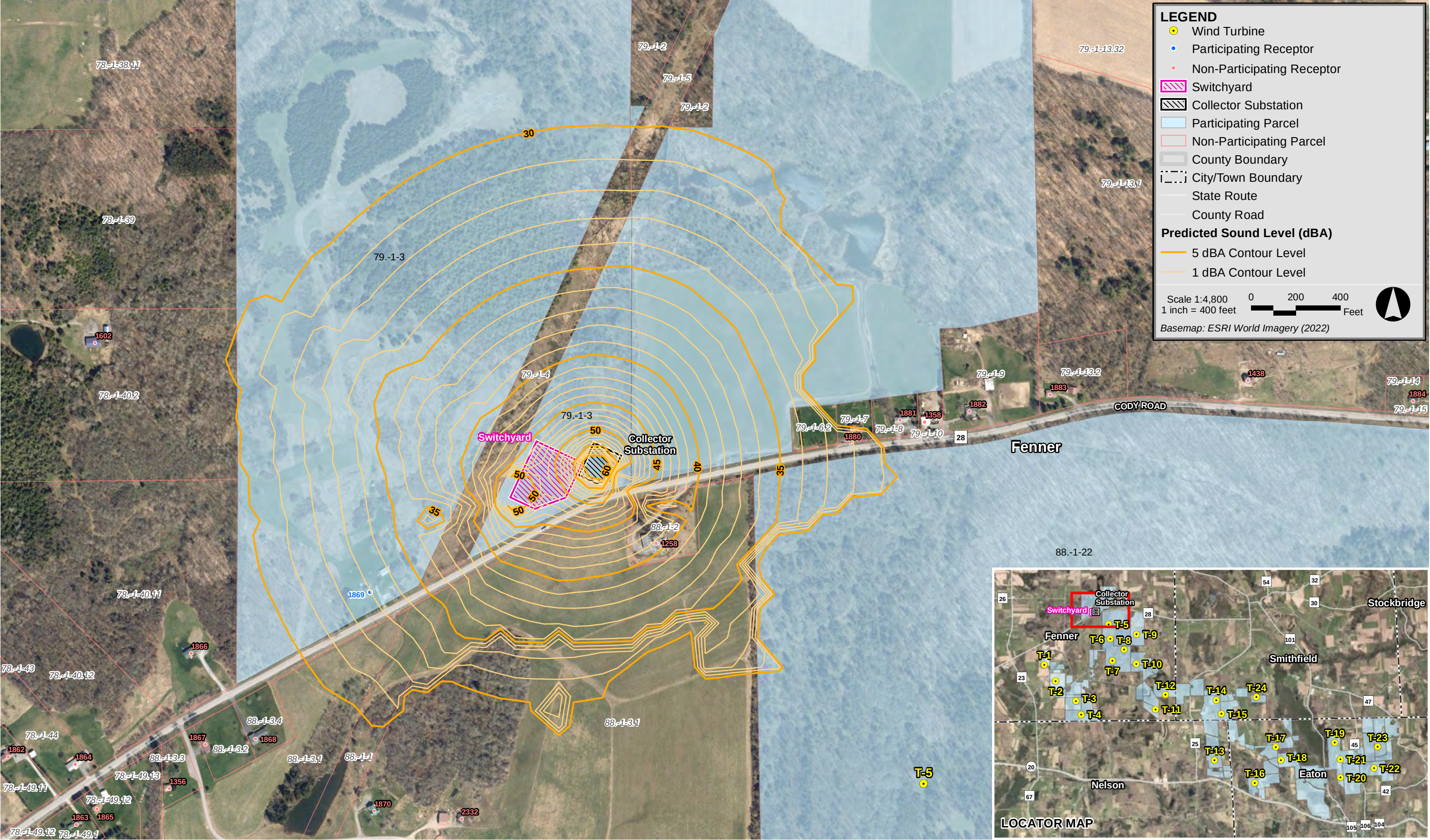
Figure 7-5.1 Collector Substation L_{eq} (1-Hr) Sound Level Modeling Results
