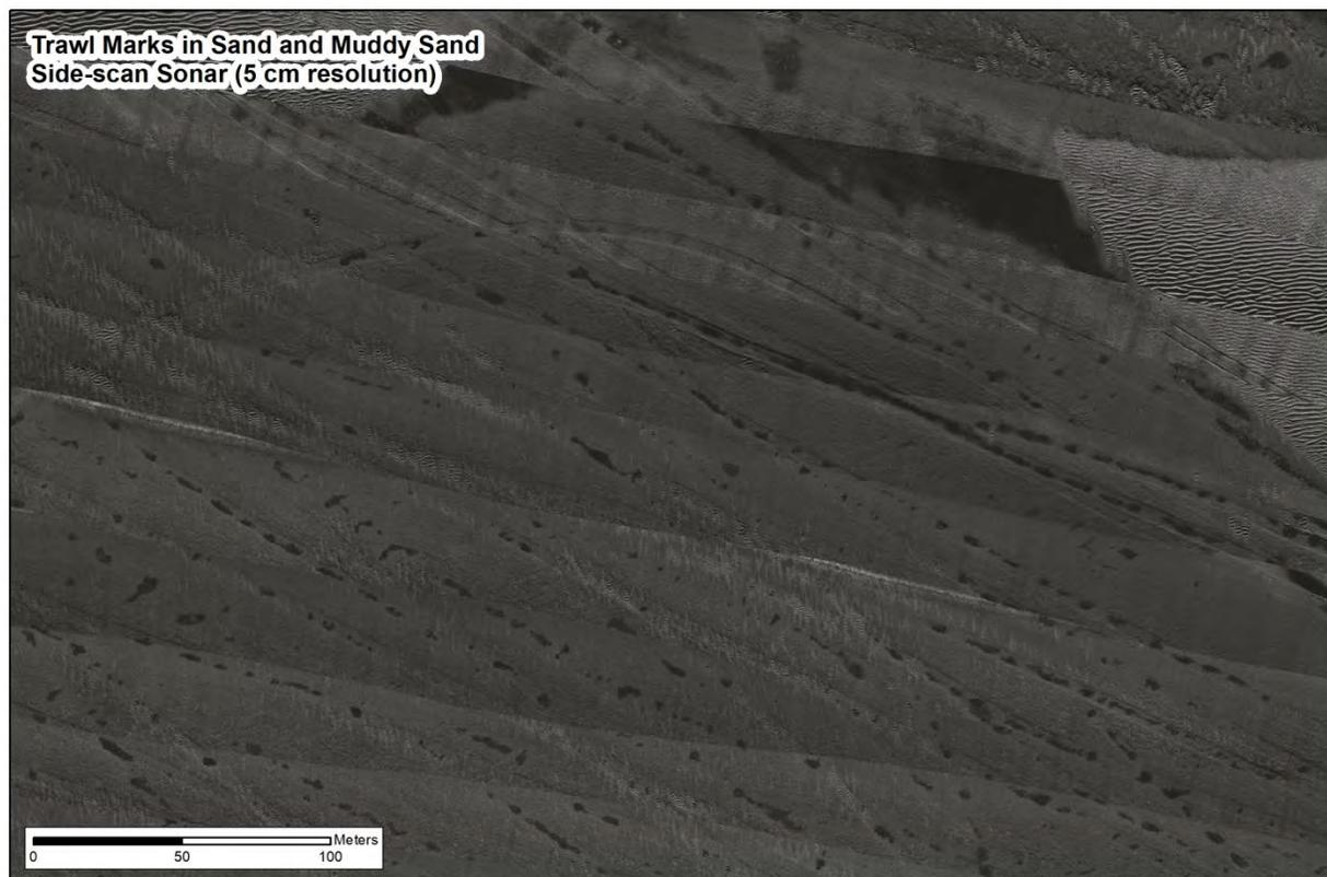
**Figure 15. Side-scan sonar data in an area of Sand and Muddy Sand at the SRW Project area, demonstrating high fishing activity as evidenced by numerous trawl marks across the sediment surface.**
