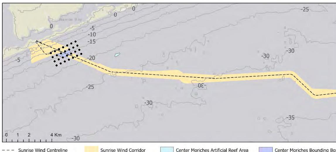
**Figure 11. Indicative diagram of the near-shore, fine-scale positioning array. The array overlaps with the SRWEC route and includes four rows of eight receivers (32 receivers total) deployed approximately 400 m apart to allow individual animals to be tracked with high spatial resolution. The exact locations of receiver deployments has not yet been determined, and will be informed by ongoing outreach efforts.**
