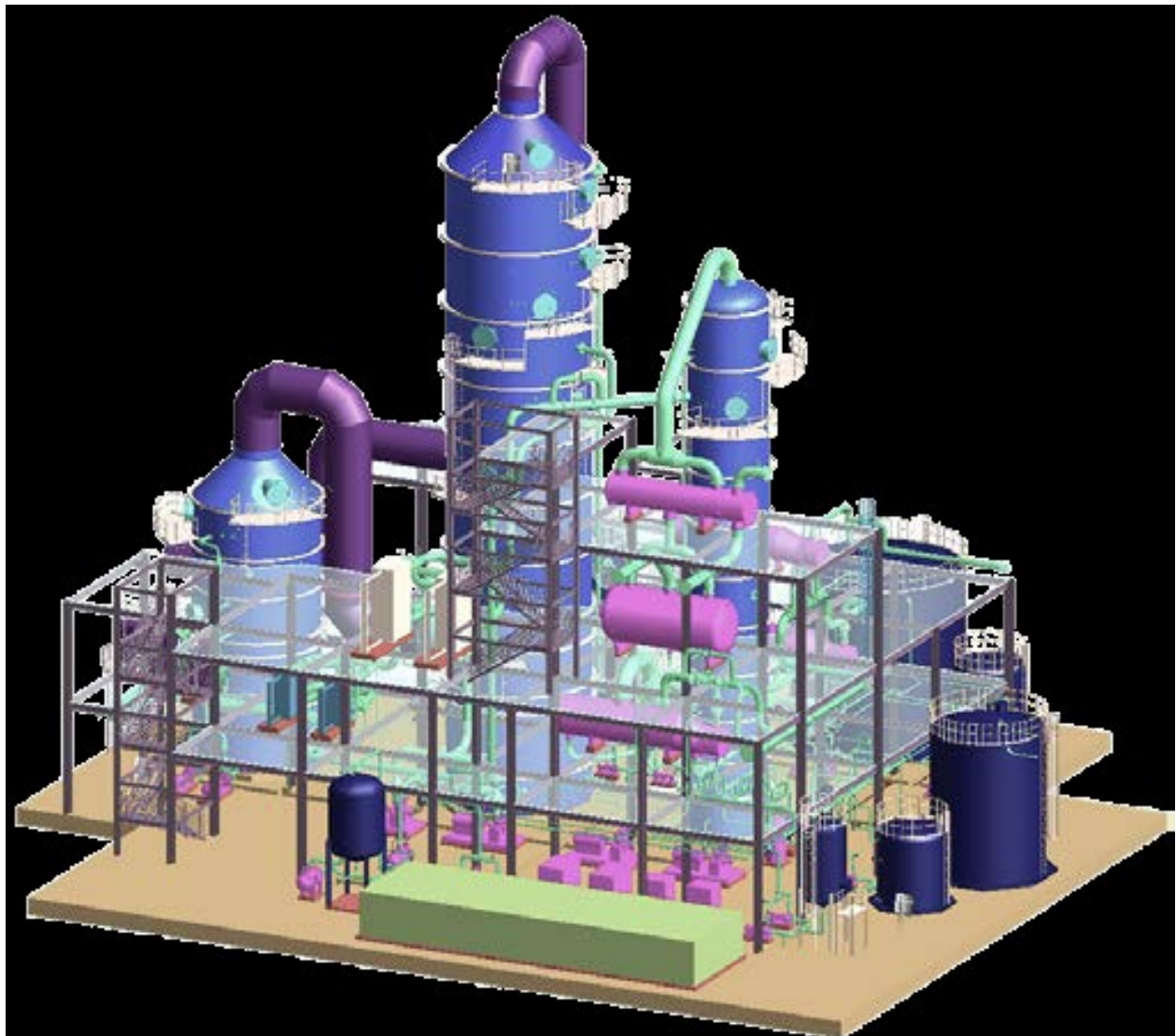
Figure 2 Image of a Solvent scrubbing facility (Courtesy of Babcock and Wilcox)
