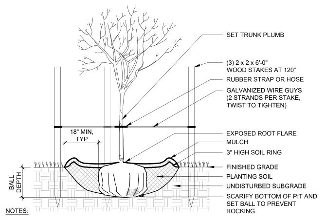
1. REMOVE BURLAP, ROPE, OR WIRE BASKET FROM TOP 1/3 OF BALL MINIMUM, CUT REMAINING PORTIONS OF ROPE OR WIRE BASKET ONCE PLANT IS IN THE FINAL POSITION IN PIT. TOP OF ROOT BALL SHALL BE SET FLUSH WITH SURROUNDING FINISHED GRADE.
