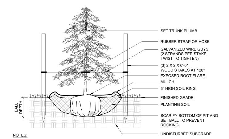
1. REMOVE BURLAP, ROPE, OR WIRE BASKET FROM TOP 1/3 OF BALL MINIMUM, CUT REMAINING PORTIONS OF ROPE OR WIRE BASKET ONCE PLANT IS IN THE FINAL POSITION IN PIT. 2. TOP OF ROOT BALL SHALL BE SET FLUSH WITH SURROUNDING FINISHED GRADE.
