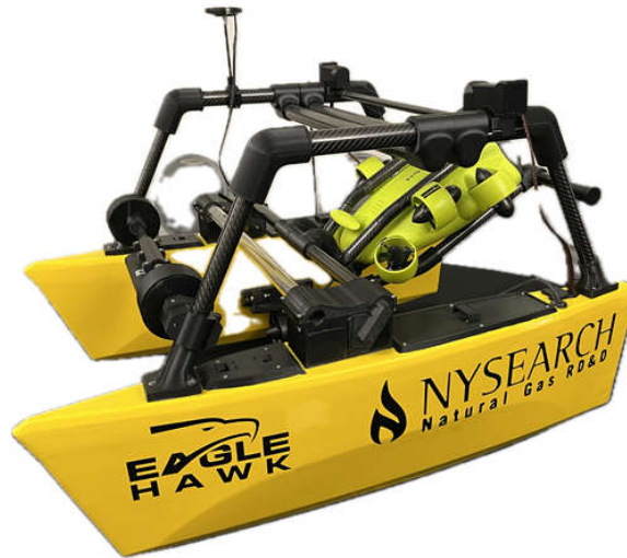
Figure 77: Aquatic Drones Perform Inspections of Submerged Pipelines
