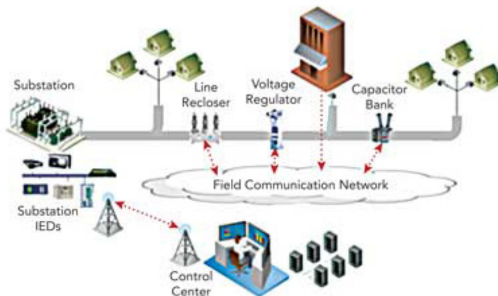
Figure 2. Illustration of a Distribution Automation System
