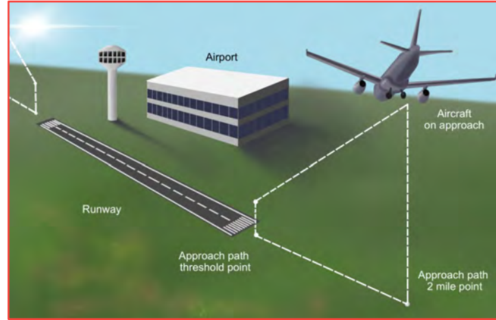
Figure 5: Illustration of a 2-mile Approach Path of Aircraft towards a Runway
