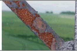
Rating 5 - "Significant Pitting" Significant pitting – loss of section clearly visible, edges feathered/thinned
