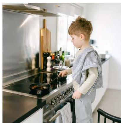
Smart and highly efficient, **electric induction stoves** cook food quickly, turn on only when a pan is placed on them, and have a smooth surface (no grates!) that cools fast.
