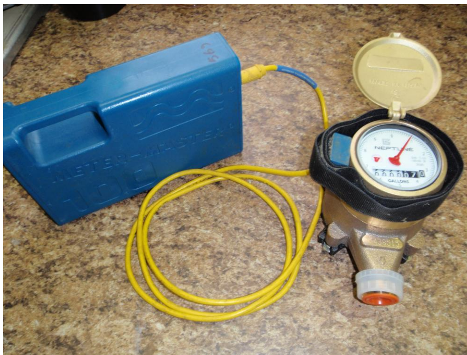
Figure 8: Meter Master 100 Flow Recorder attached to residential water meter
