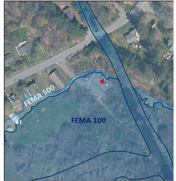
Figure 16. Summitville substation (red point) with the FEMA 100- and 500-year floodplains overlaid.
