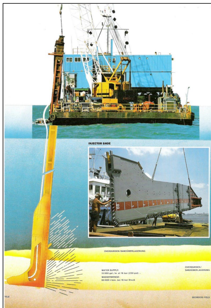
Figure 6-6 Illustration of vertical injector deployed from cable lay barge ( www.miahtrenchers.com )
