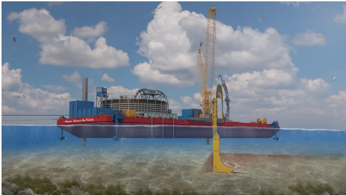
Figure 2: Cable Lay Barge with Vertical Injector (VI)
