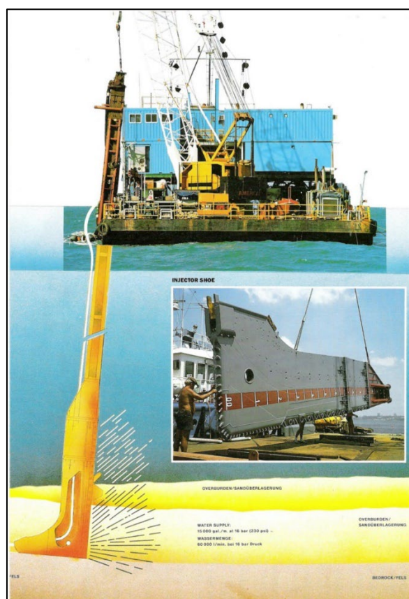
Figure 5-1 Illustration of vertical injector deployed from cable lay barge ( www.miahtrenchers.com )
