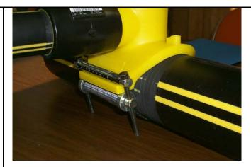
Test proper functioning of the micropressure sensors by pushing down on them individually, verifying the fusion end cycle. Remove protective caps from terminal wells and connect fusion control box leads to fitting. Ensure leads are connected properly.
