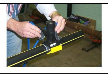
Activate the fusion cycle .When the fusion is complete, the fusion end light on the control box will light. At this time, wait an additional 30 second before removing leads. NOTE: If fusion cycle is interrupted for any reason, the recommended cooling time (table) must be waited before re-starting the fusion process over.
