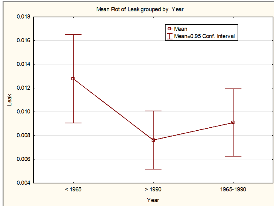
Figure 46. Mean Plot of Leak Indication vs. Installation Year
