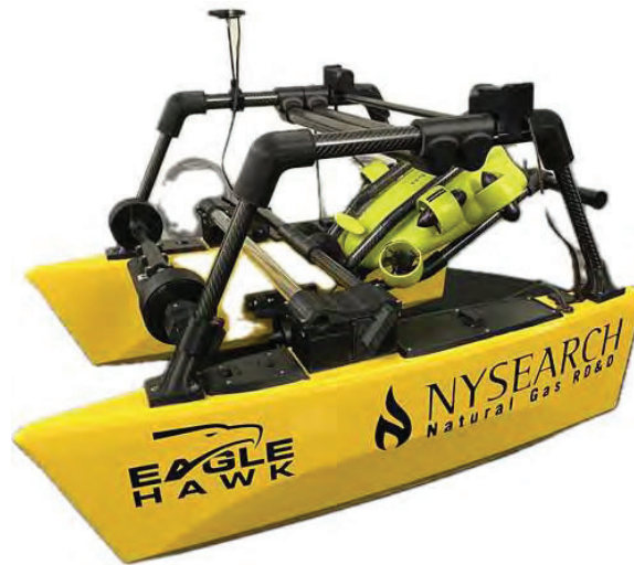
Figure 47: Aquatic Drones Perform Inspections of Submerged Pipelines
