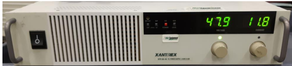
DC power supply for fans
