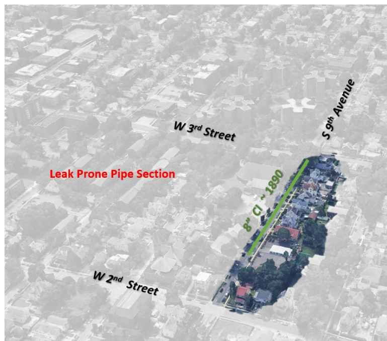
Figure 4: Leak Prone Pipe Section of Mount Vernon Project
