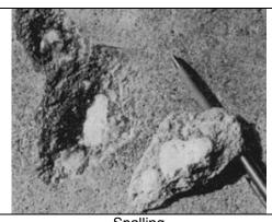
Spalling Development of fragments Delamination Degradation of steel/concrete interface
