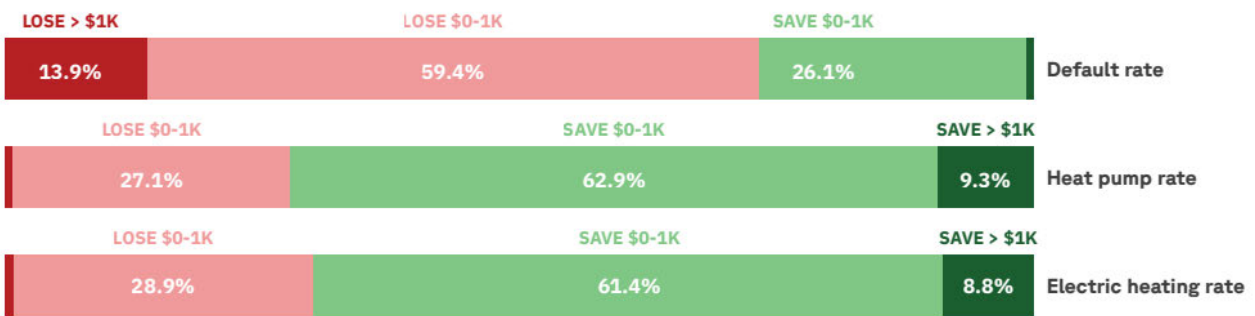
Figure 8. Change in total annual energy bills — natural gas homes switching to a heat pump: default rate vs. electric heating rate (Statewide). Assumes 40% of LMI households are enrolled in utility energy affordability programs before and after switching to a heat pump.
