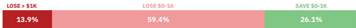
Figure 2. Change in total annual energy bills (electricity + natural gas) for natural gas-heated households that switch to heat pumps (NY, statewide). Assumes 40% of LMI households are enrolled in the utilities’ energy affordability program before and after switching to a heat pump.
