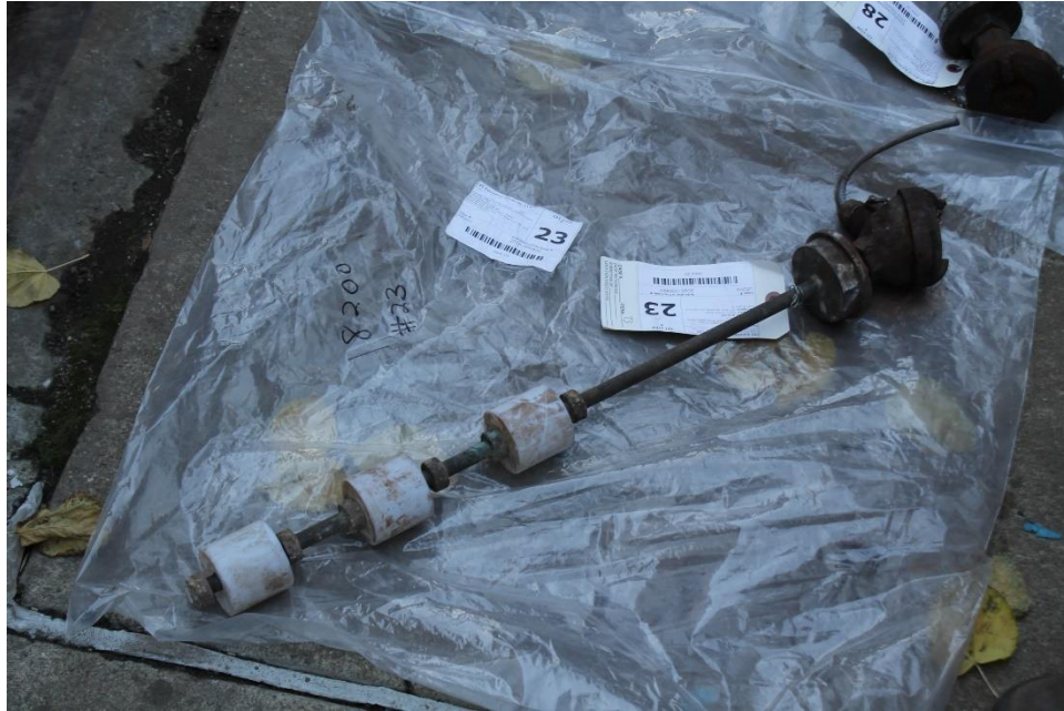
Figure 14 - Photo of Manhole Float, Taken by Staff
