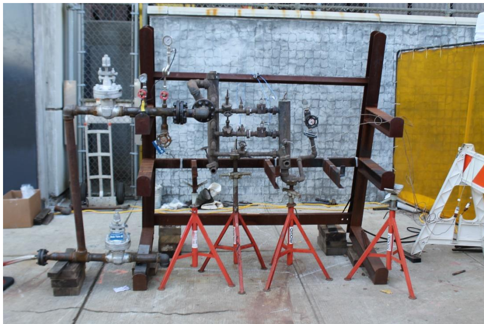
Figure 15 - Photo of Trap Assembly During Testing on November 1 st , 2018, Taken by Staff
