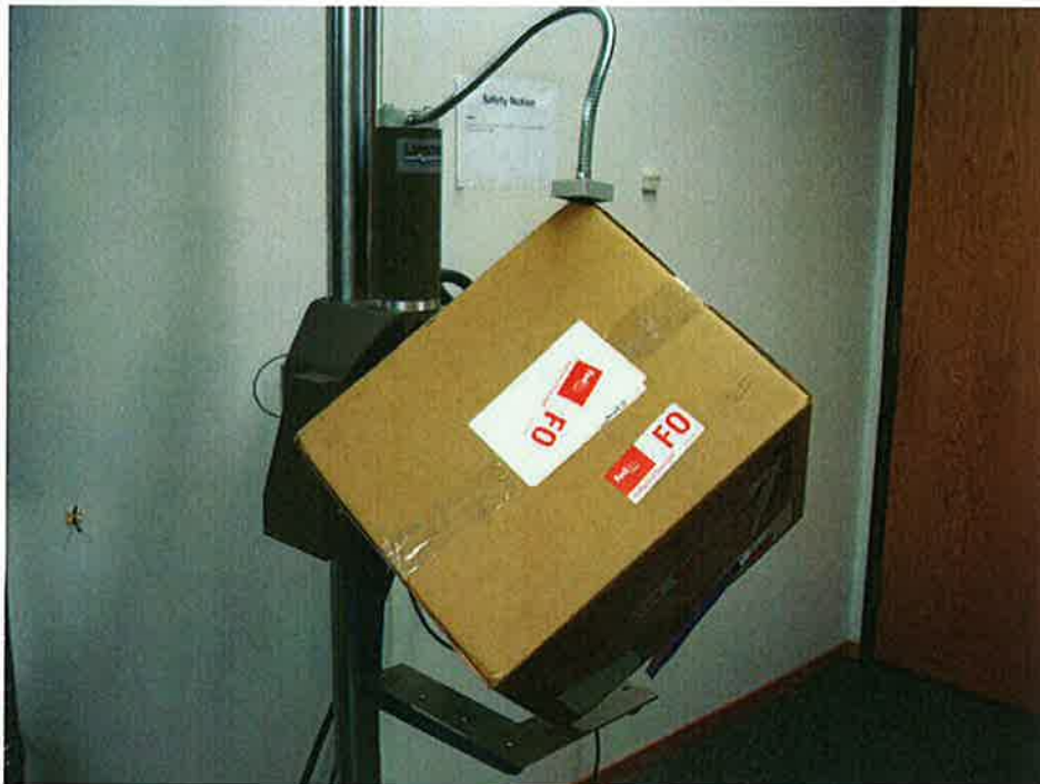
Figure 24: Shipping container (Seam Split – 2-3-5 corner)
