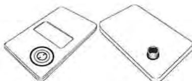
Pit Lid Housing Inserted Through Pit Lid (Top View)
