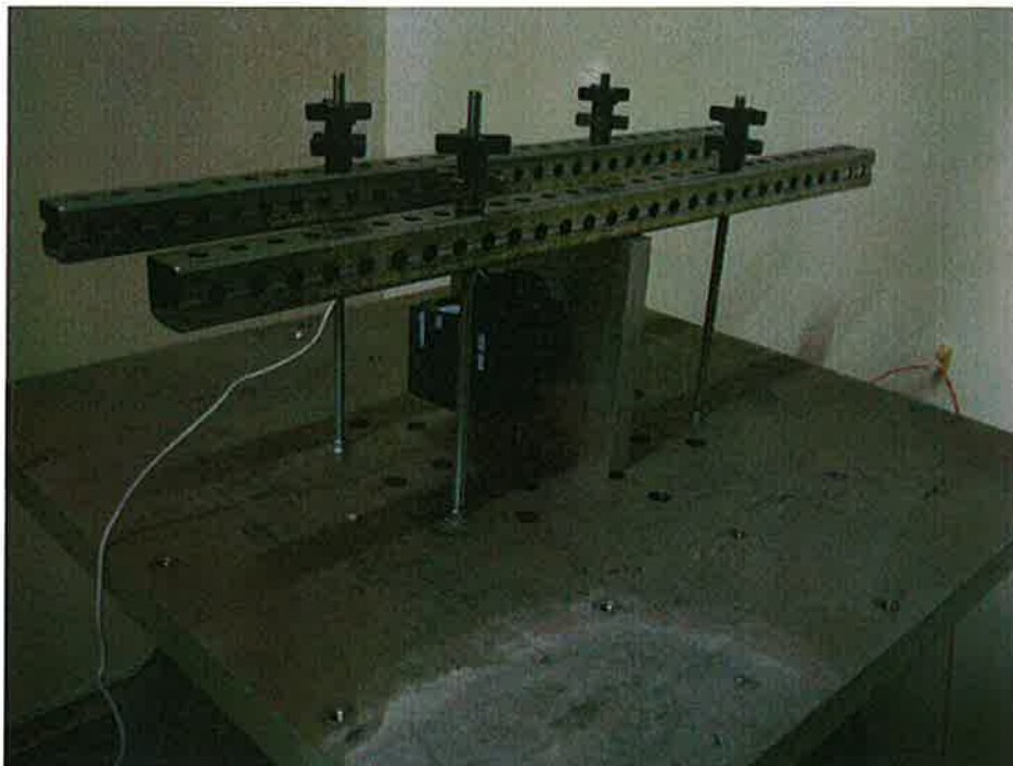
Figure 19: NA 2 WAY Reliability –TC–10.4 Operational Vibration (Y axis)
