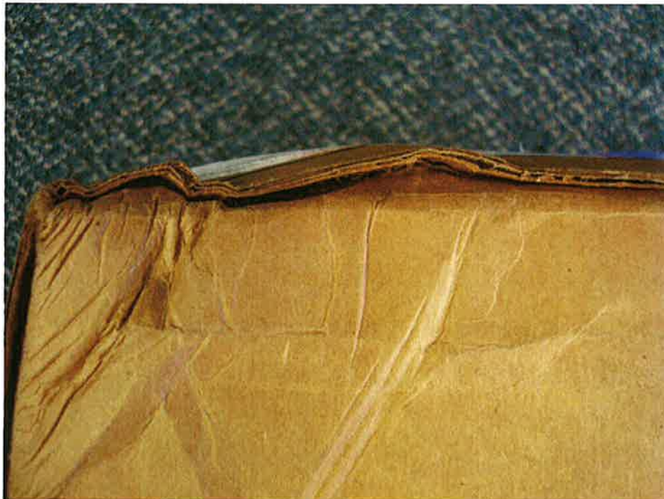
Figure 24: Shipping container (Seam Split – 2-3-5 corner)
