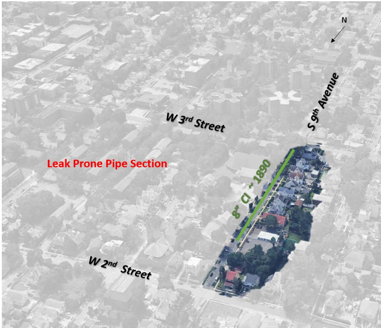
Figure A.5. Leak Prone Pipe Section of Mount Vernon Project
