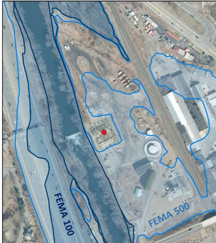
Figure 1. Hillburn Substation yard (red dot) is located next to the Ramapo River and within the FEMA 500-year flood plain extent.
