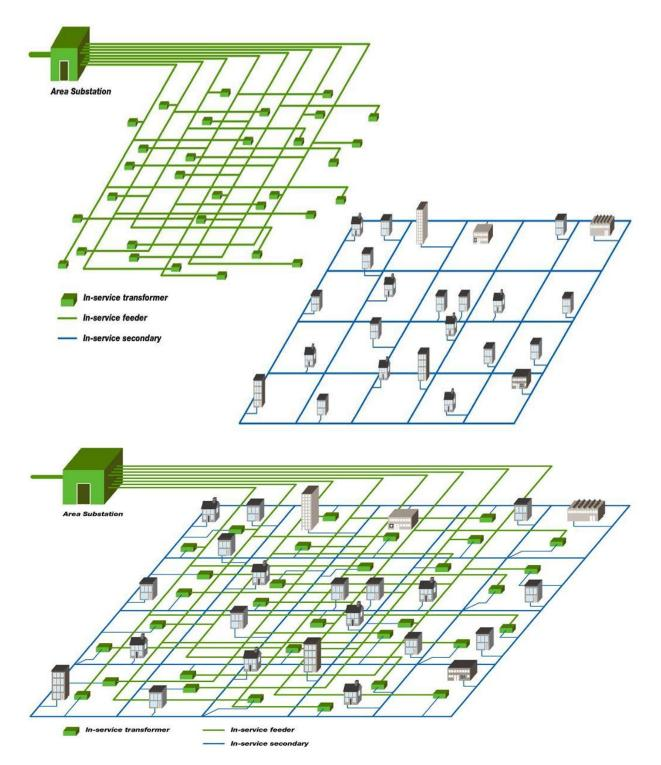
The network is designed to have two distribution feeders (13kV or 27kV) out of service without interrupting customers – N-2 design. The system is designed to withstand two feeders out of service during the forecasted summer peak load without interrupting service to customers.
