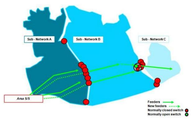
In the diagram, three sub-networks are established. Network feeders continue to run throughout the network, with sectionalizing switches at the sub-network boundaries to isolate each sub-network. Two
