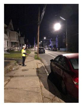
Figure 2. National Grid employee Chong Lin measured light output using a lux meter on Congress Street.
