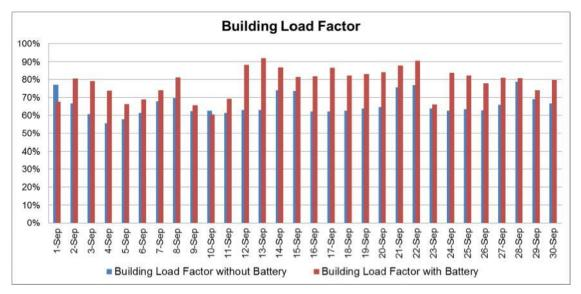
Figure 3. Building load factor w and w/o presence of battery
