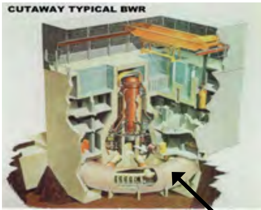
A look inside a boiling water reactor, like FitzPatrick Torus
