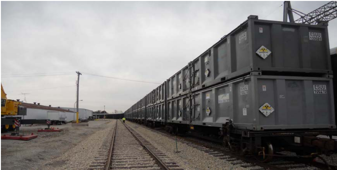
Photo 9: Intermodal Containers for Transporting Radioactive Waste
