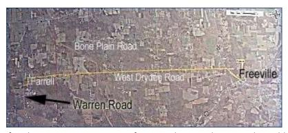
The Dominion Transmission, Inc. (DTI) interstate pipeline covers 7,800 miles of natural gas transmission pipes in six states. The proposed project would hook up to the pipeline in Freeville, north for a short distance along NYS Route 38 along West Dryden and Farrell Roads to the Warren Road area of Lansing, totaling about seven miles of 10" steel pipe.
