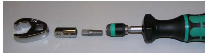
11-29 inch-pound torque setting screwdriver with Phillips tip made by Wera
