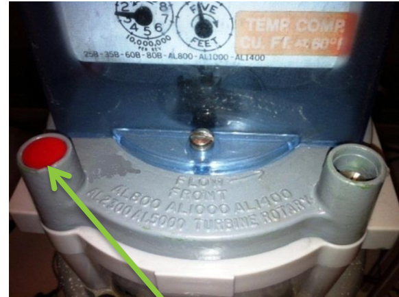
Index assembly with tamper cup uses a tamper seal
