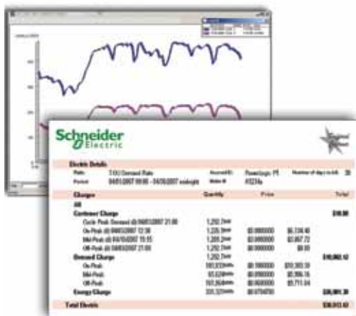
PowerLogic EM4800 on-site software or web-hosted services can be used for bill preparation, energy analysis, and data export to other applications or to billing services.
