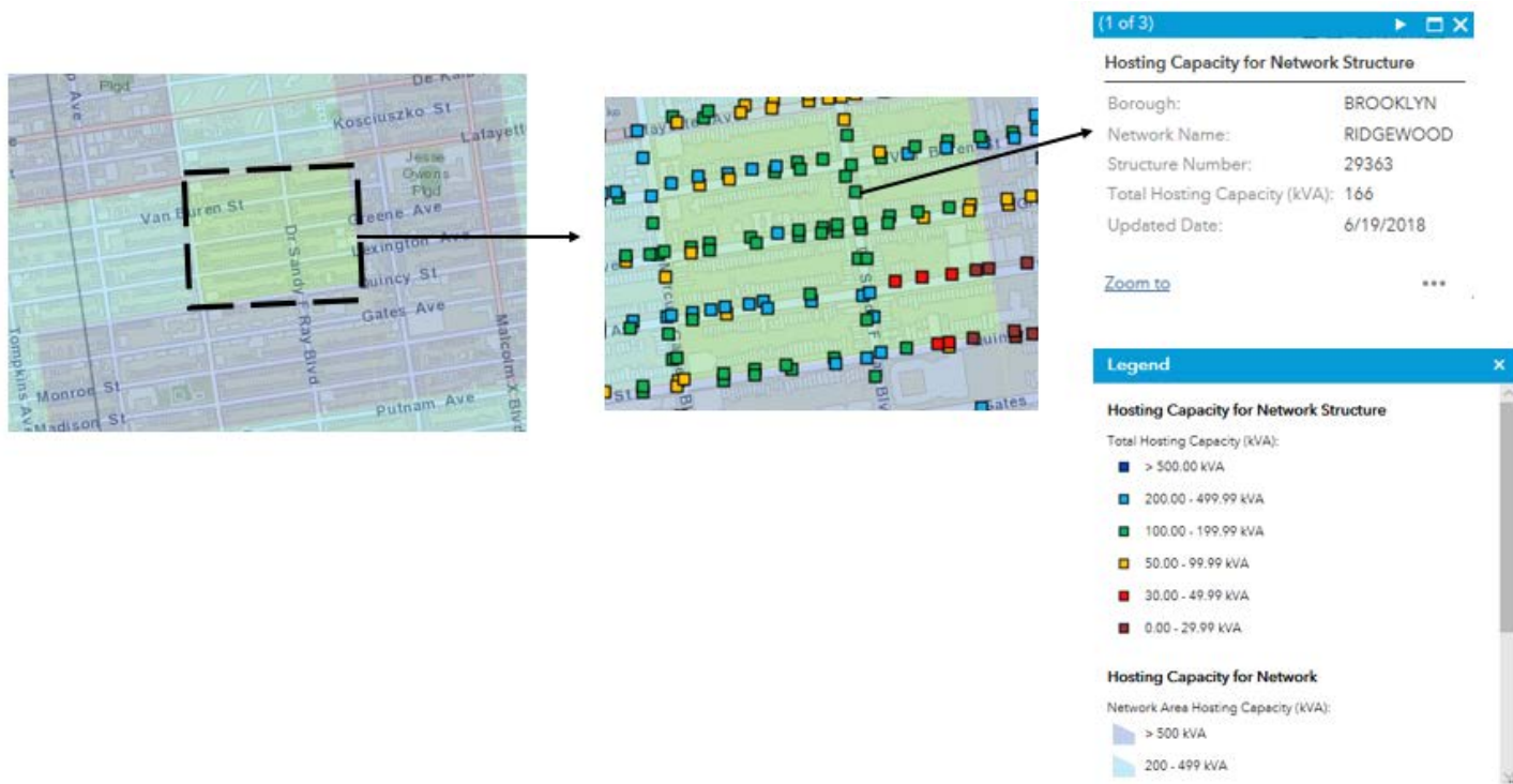
Figure 46: Hosting Capacity for Individual Network Structures
