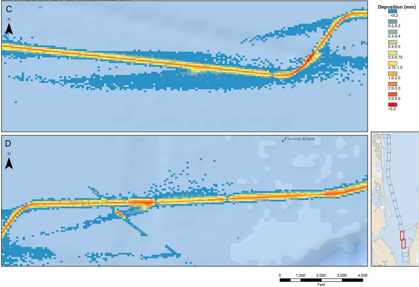
**Figure 15.3 Model Total Sediment Deposition Thickness**
