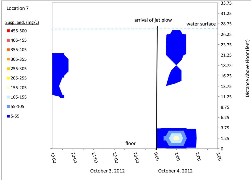
**Figure 14.7 Model Water Column Suspended Sediment Concentration Over Time**
