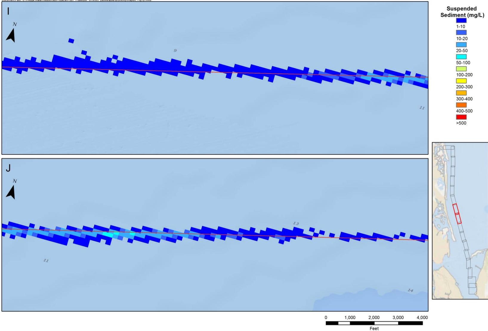
**Figure 12.6 Model Maximum Suspended Sediment Concentrations**
