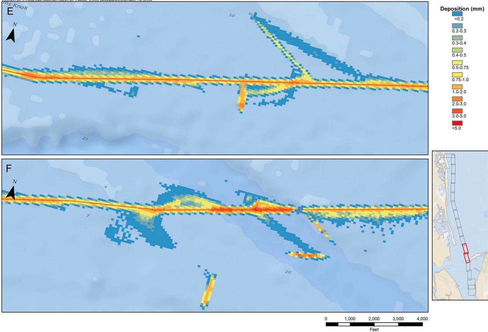
**Figure 15.4 Model Total Sediment Deposition Thickness**
