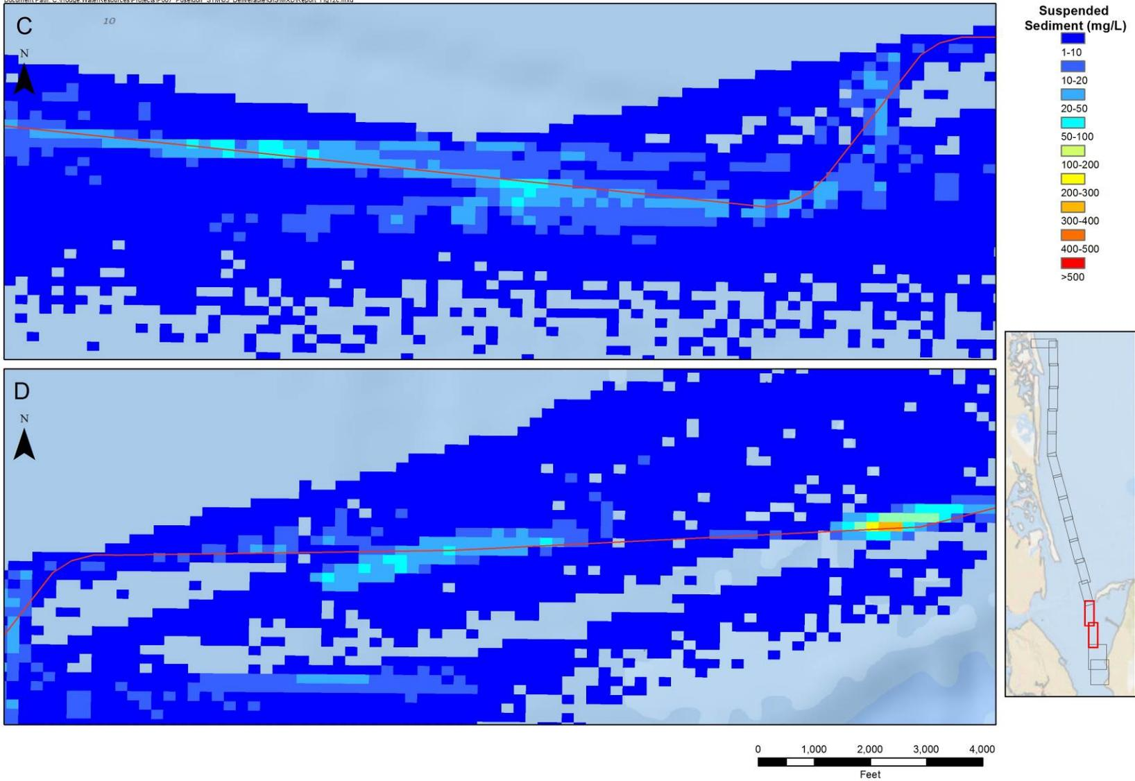
**Figure 12.3 Model Maximum Suspended Sediment Concentrations**
