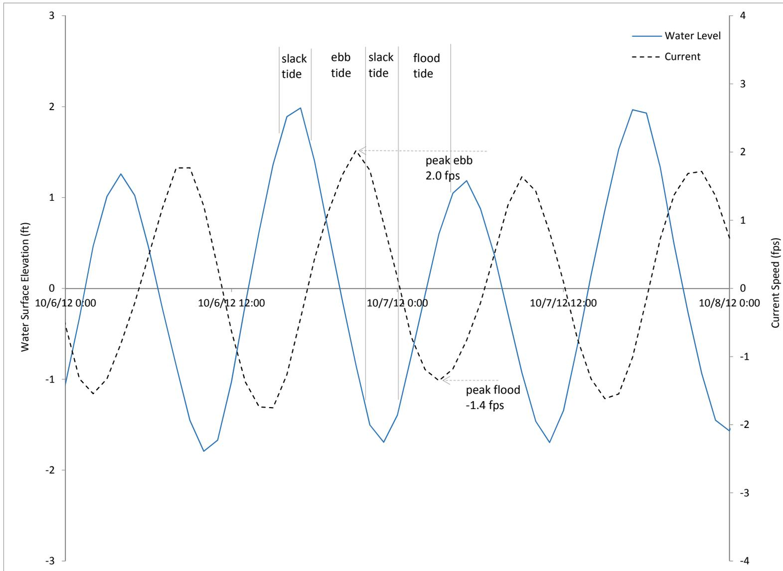
**Figure 3 Typical Hydrodynamic Model Tide and Current Cycles**
