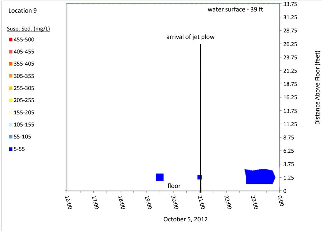
**Figure 14.9 Model Water Column Suspended Sediment Concentration Over Time**
