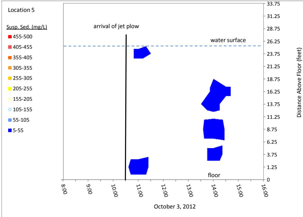
**Figure 14.5 Model Water Column Suspended Sediment Concentration Over Time**
