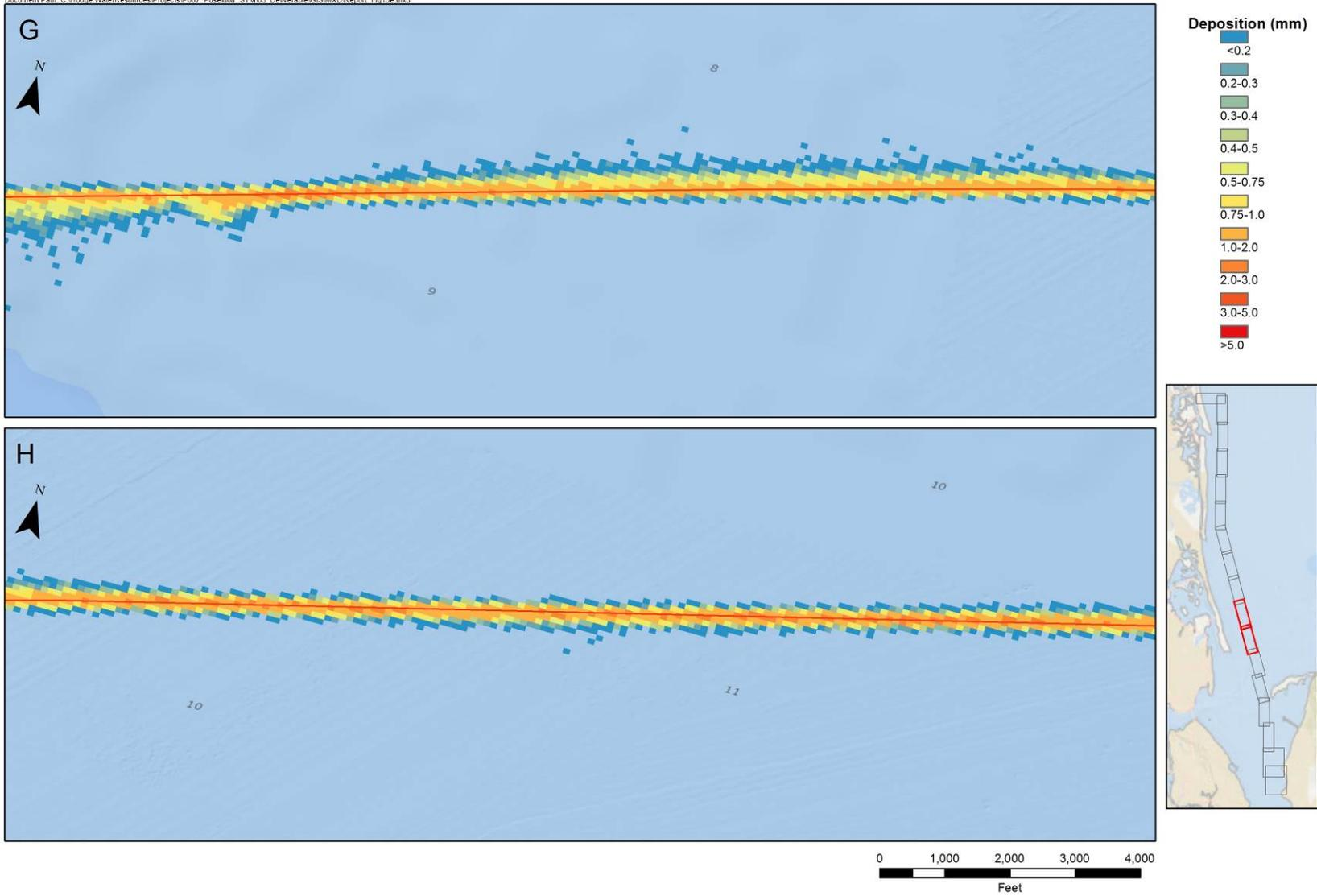
**Figure 15.5 Model Total Sediment Deposition Thickness**
