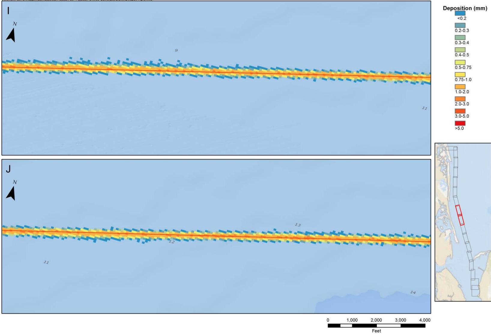
**Figure 15.6 Model Total Sediment Deposition Thickness**
