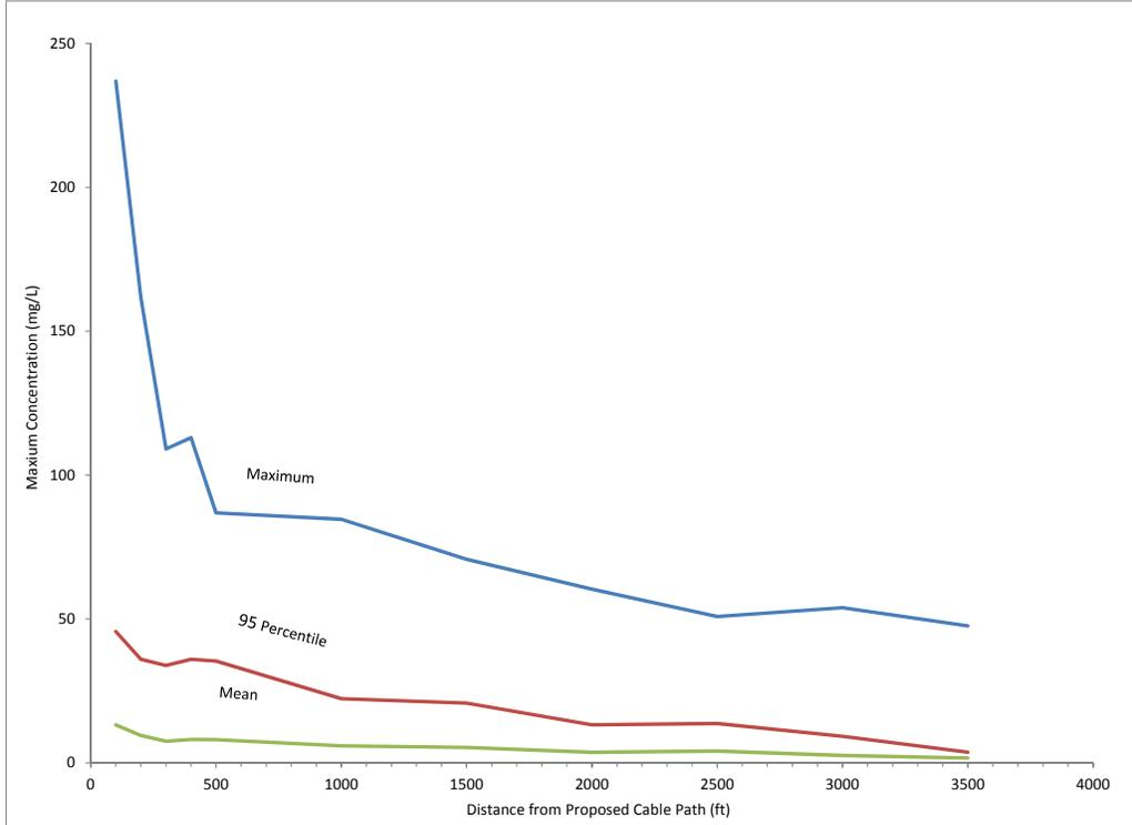
**Figure 16 Suspended Sediment Concentration Excursions from Cable Route**
