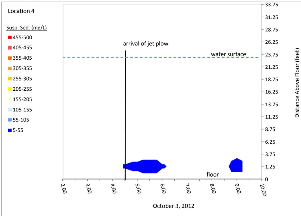
**Figure 14.4 Model Water Column Suspended Sediment Concentration Over Time**
