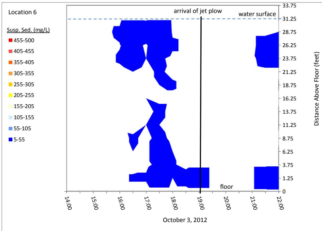
**Figure 14.6 Model Water Column Suspended Sediment Concentration Over Time**
