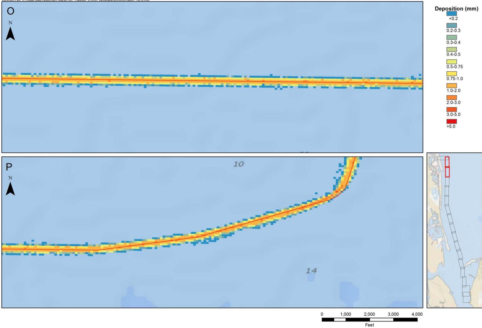
**Figure 15.9 Model Total Sediment Deposition Thickness**
