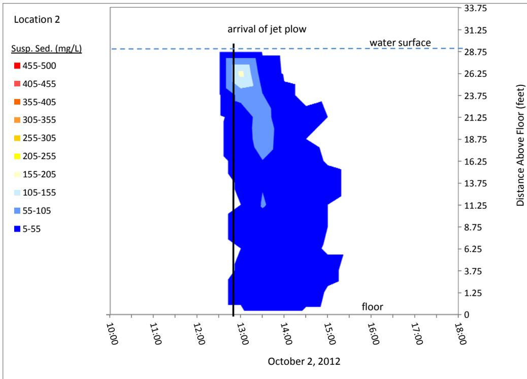
**Figure 14.2 Model Water Column Suspended Sediment Concentration Over Time**
