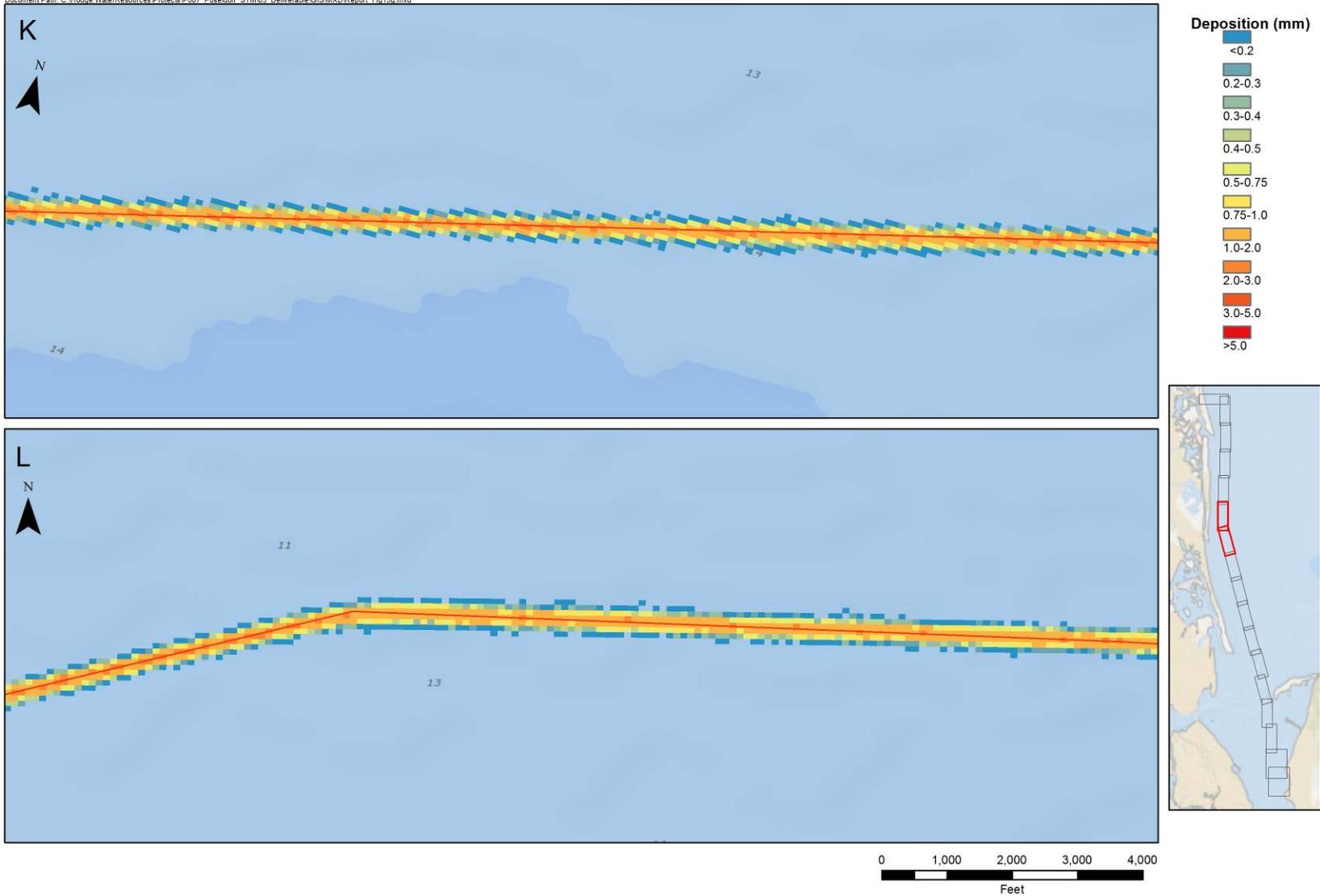
**Figure 15.7 Model Total Sediment Deposition Thickness**
