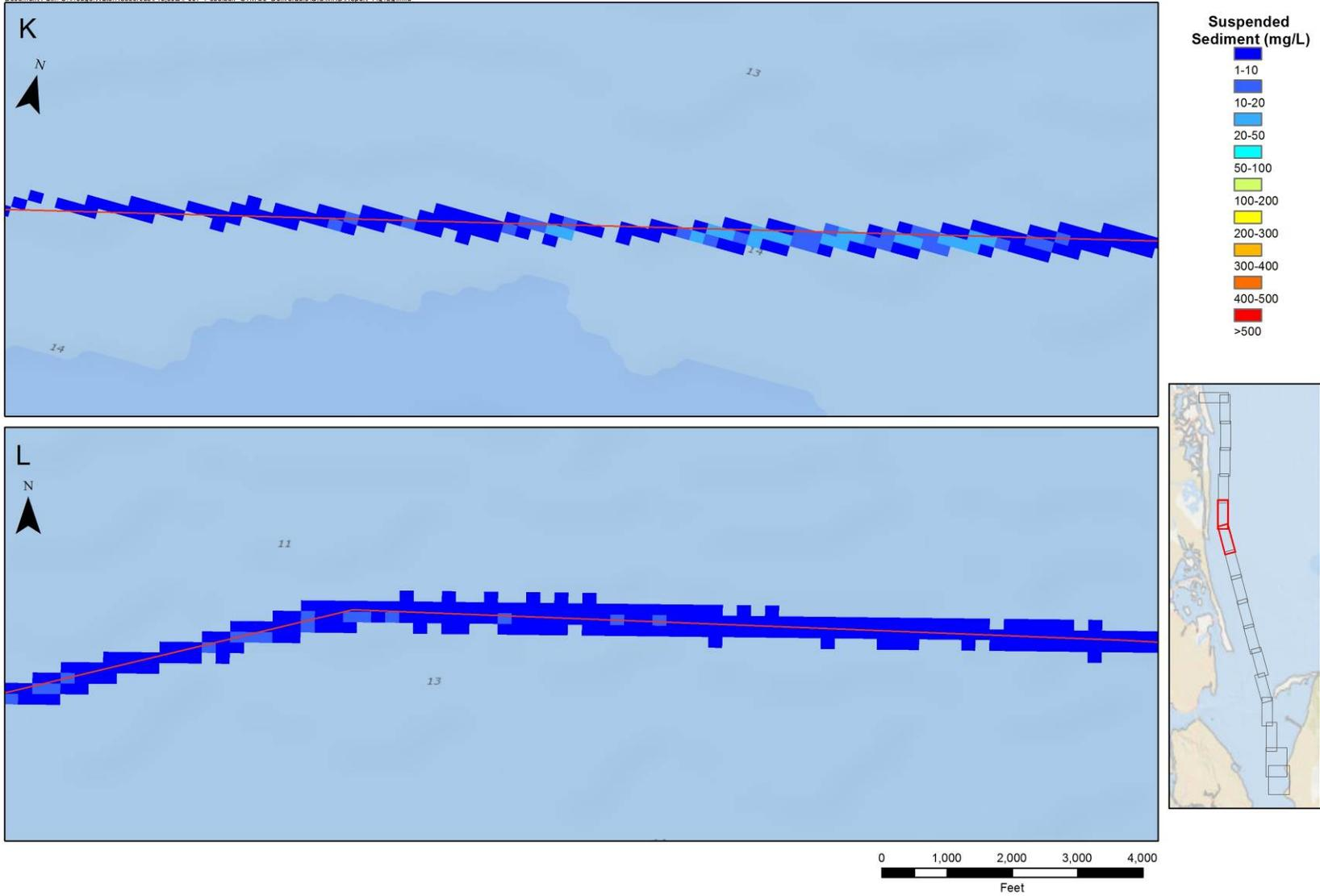
**Figure 12.7 Model Maximum Suspended Sediment Concentrations**
