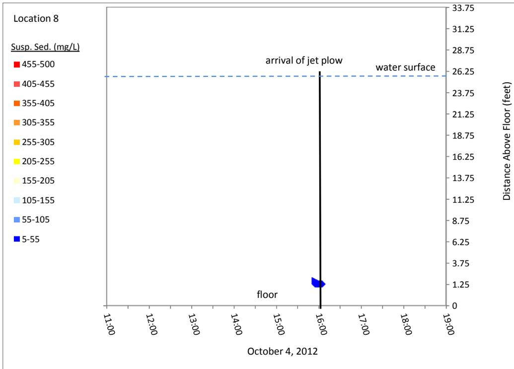
**Figure 14.8 Model Water Column Suspended Sediment Concentration Over Time**
