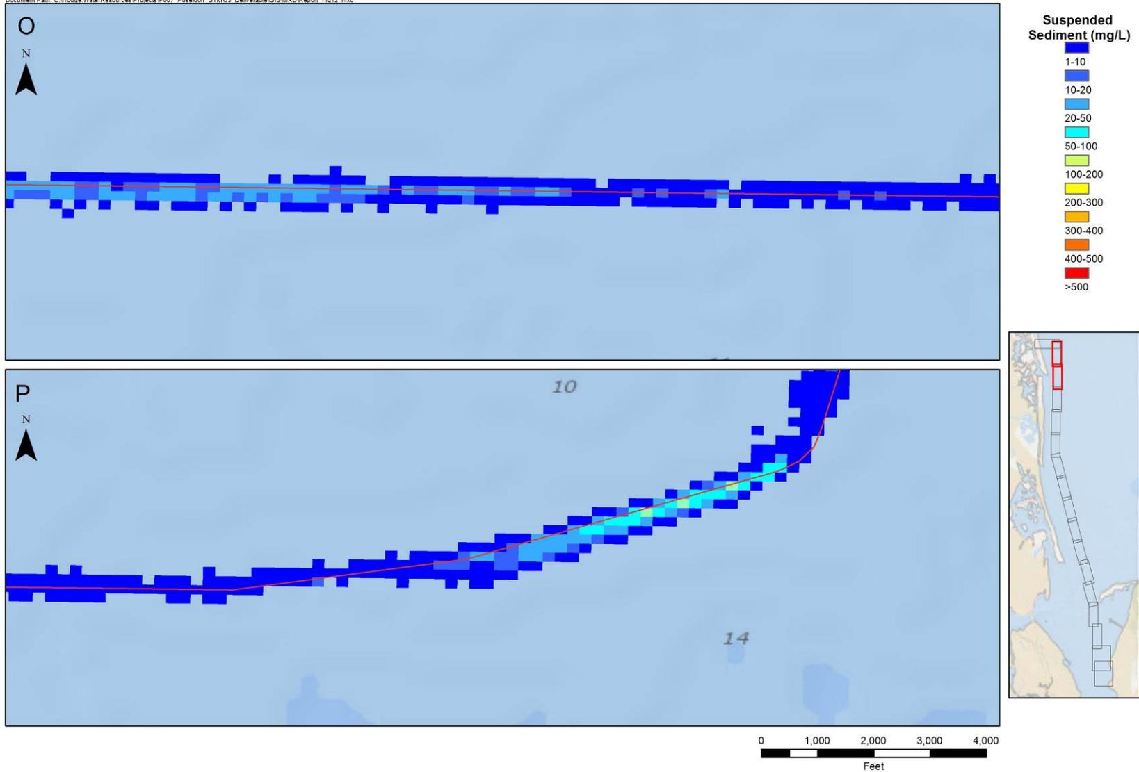
**Figure 12.9 Model Maximum Suspended Sediment Concentrations**
