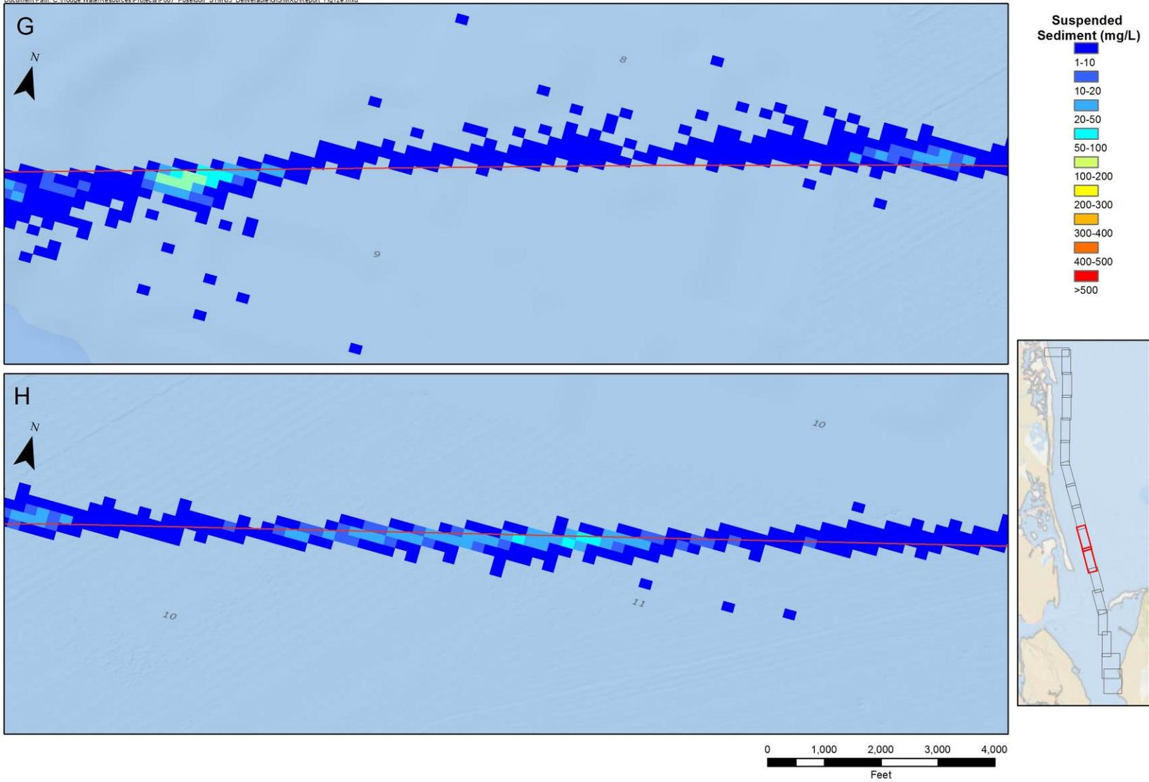
**Figure 12.5 Model Maximum Suspended Sediment Concentrations**
