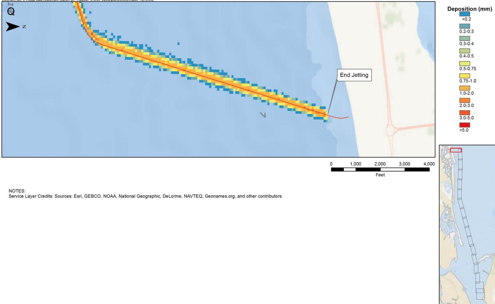
**Figure 15.10 Model Total Sediment Deposition Thickness**
