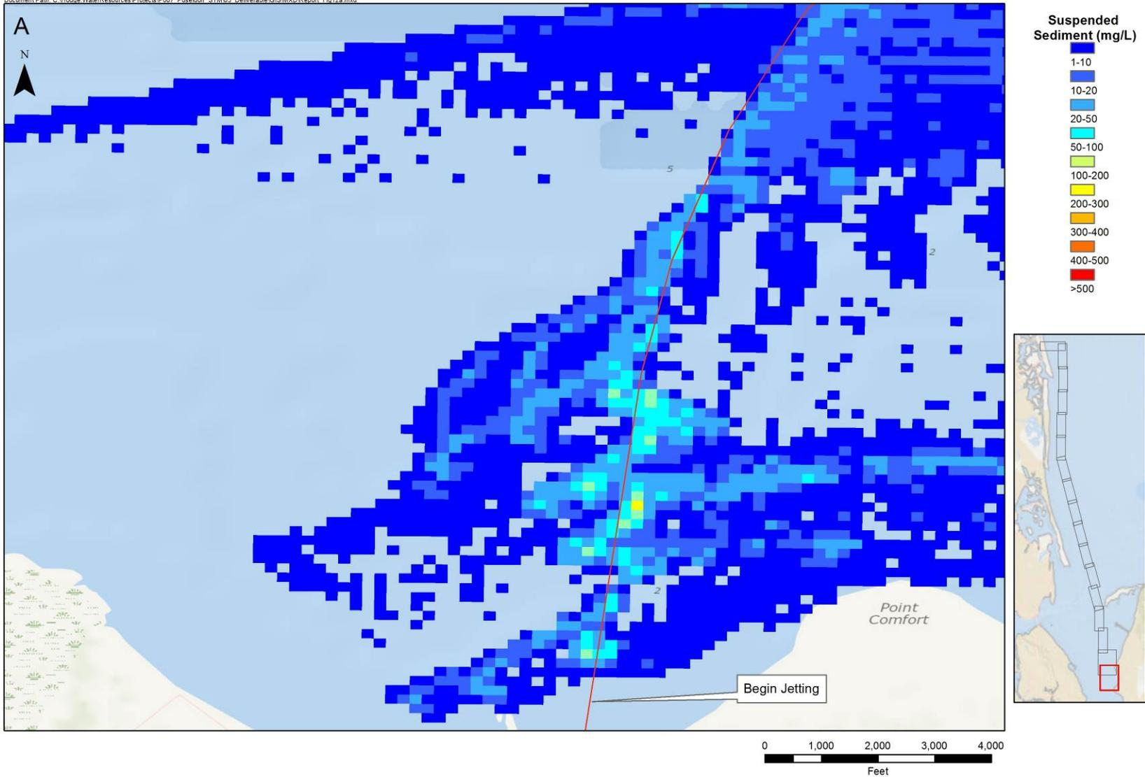
**Figure 12.1 Model Maximum Suspended Sediment Concentrations**
