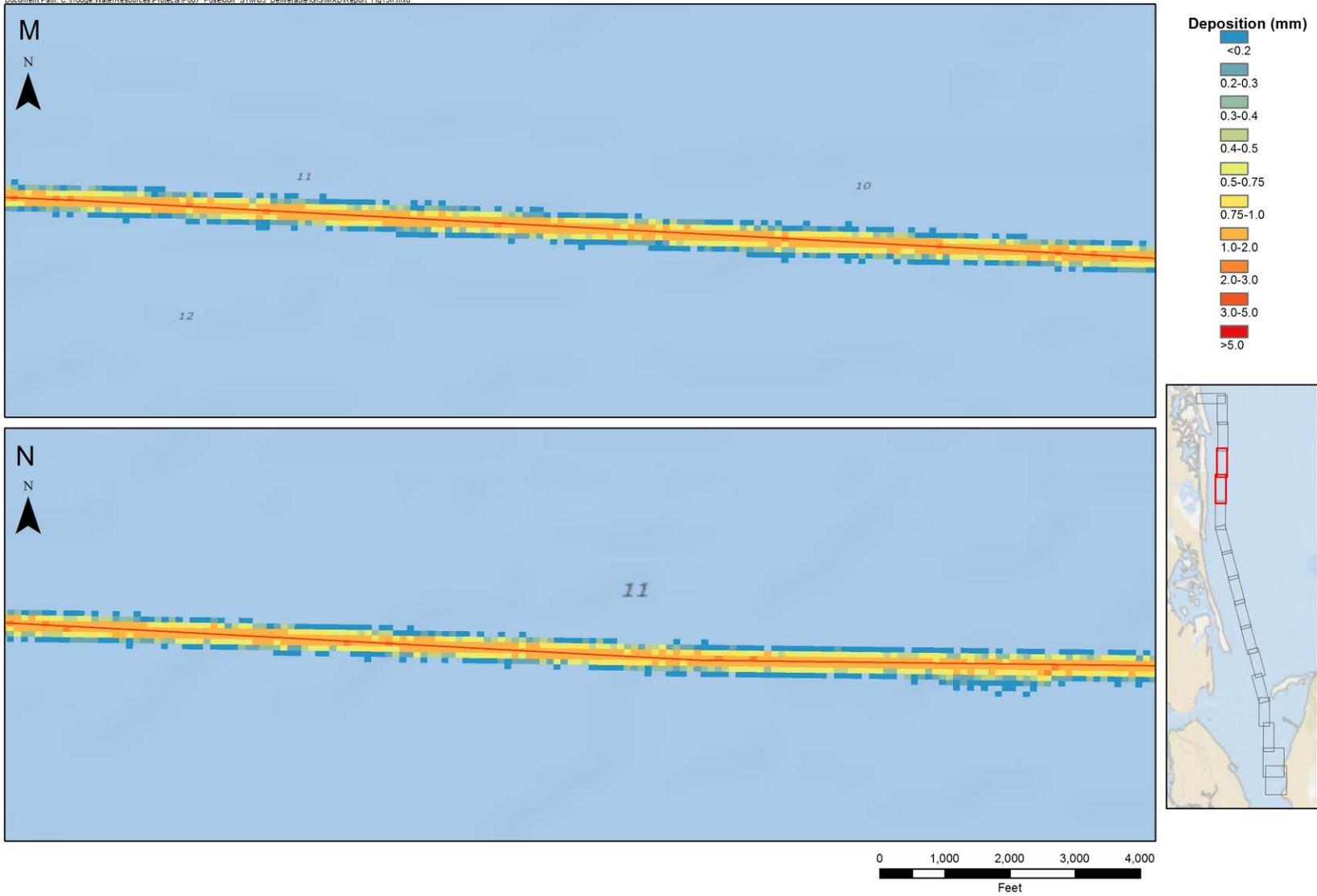
**Figure 15.8 Model Total Sediment Deposition Thickness**
