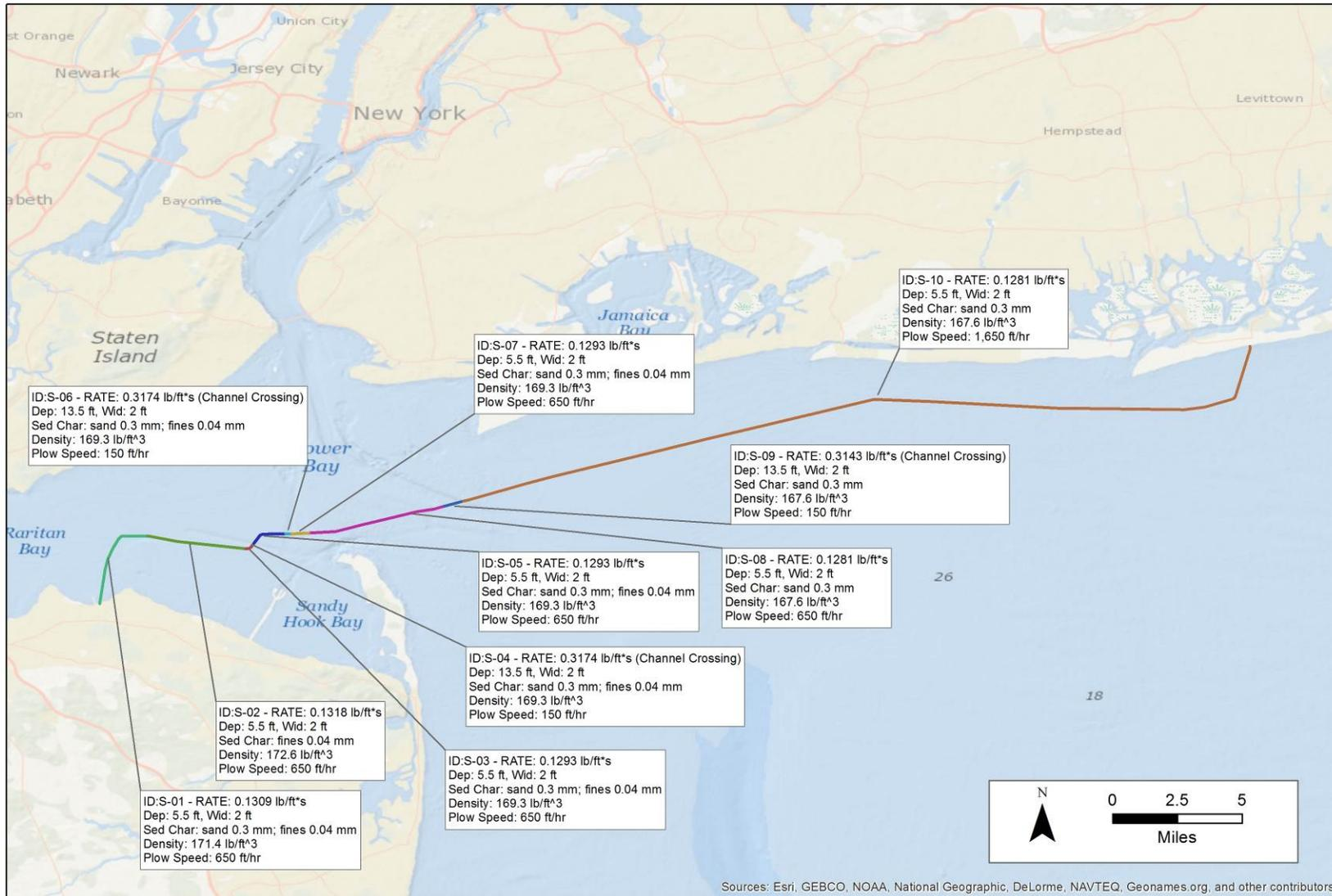
**Figure 10 Sediment Dispersion Model Input Segments**
