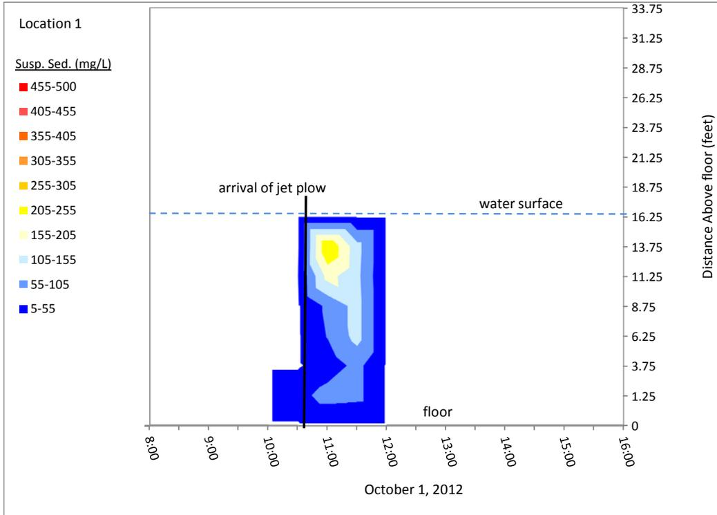
**Figure 14.1 Model Water Column Suspended Sediment Concentration Over Time**
