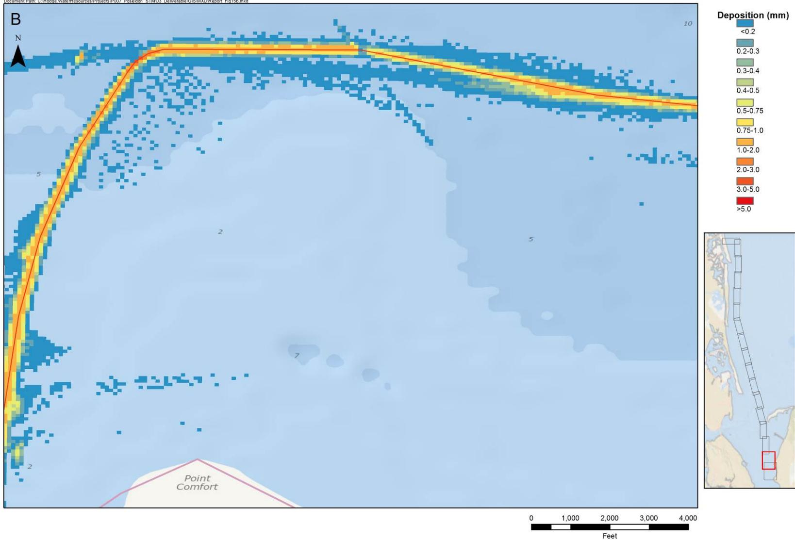
**Figure 15.2 Model Total Sediment Deposition Thickness**
