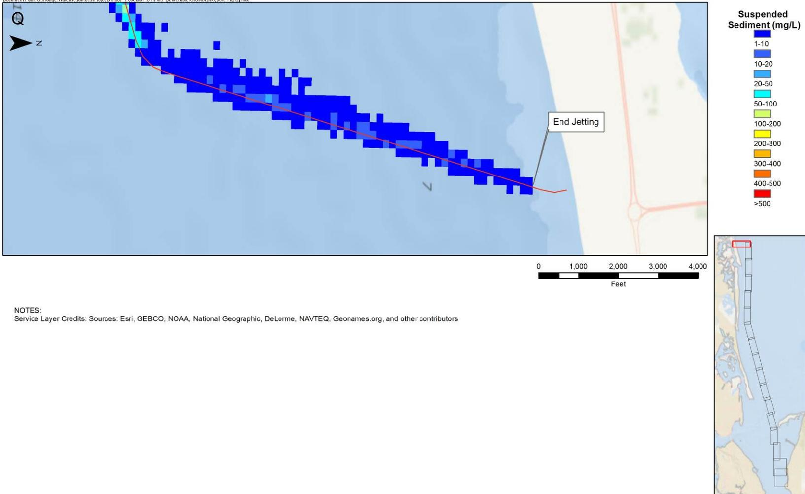
**Figure 12.10 Model Maximum Suspended Sediment Concentrations**
