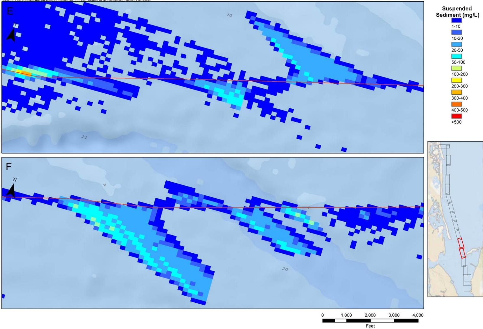
**Figure 12.4 Model Maximum Suspended Sediment Concentrations**
