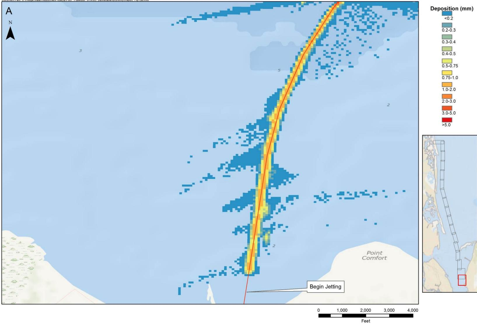
**Figure 15.1 Model Total Sediment Deposition Thickness**
