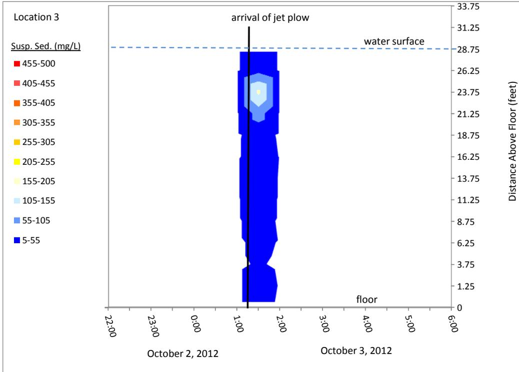
**Figure 14.3 Model Water Column Suspended Sediment Concentration Over Time**
