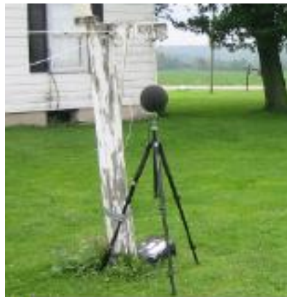
Figure 21. Rion Windscreen in use at a Stony Creek Ambient Noise Monitoring Site
