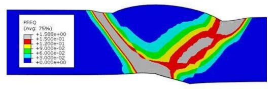
Contour of plastic strain. Note that the plastic strain in the HAZ is much higher than that in the pipe and upper fill passes.
