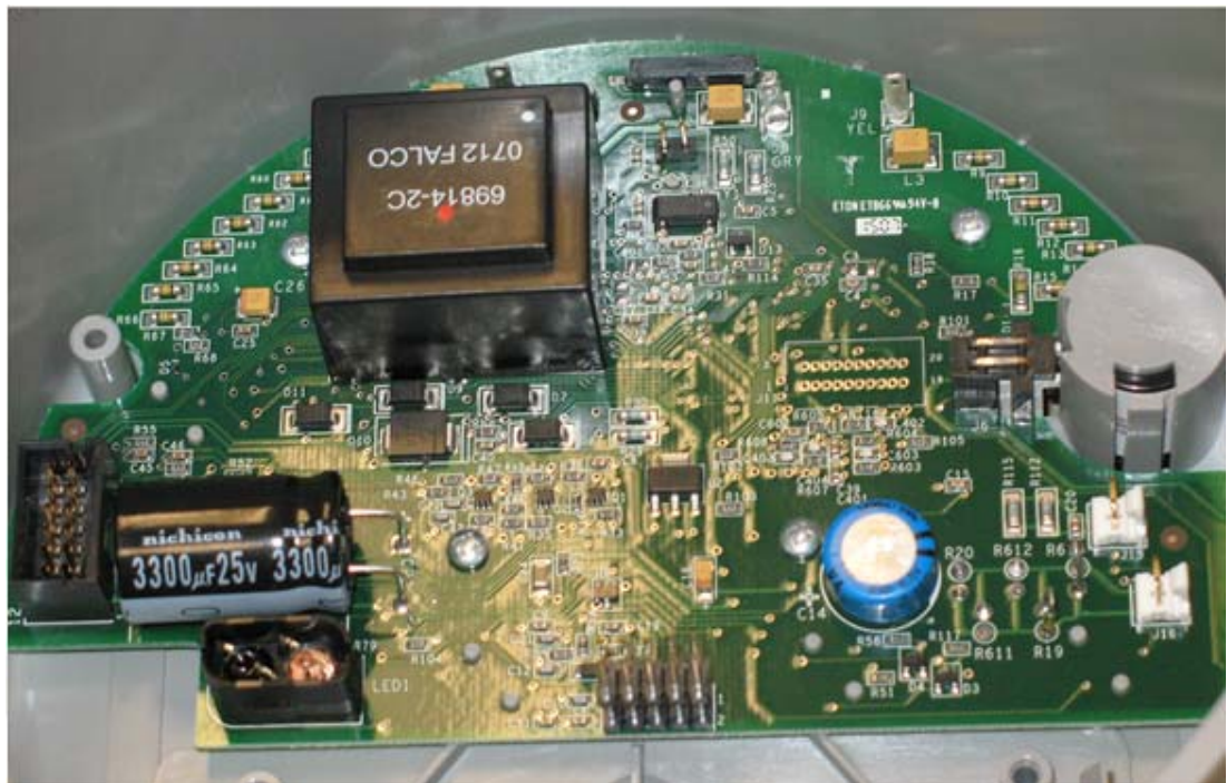
Meter board inside housing
