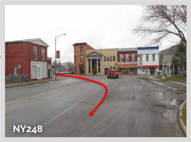
Intersection of NY36 and NY248 in Canisteo measured 135ft, however has limitation. 67.2m Blade CANNOT travel through here.
