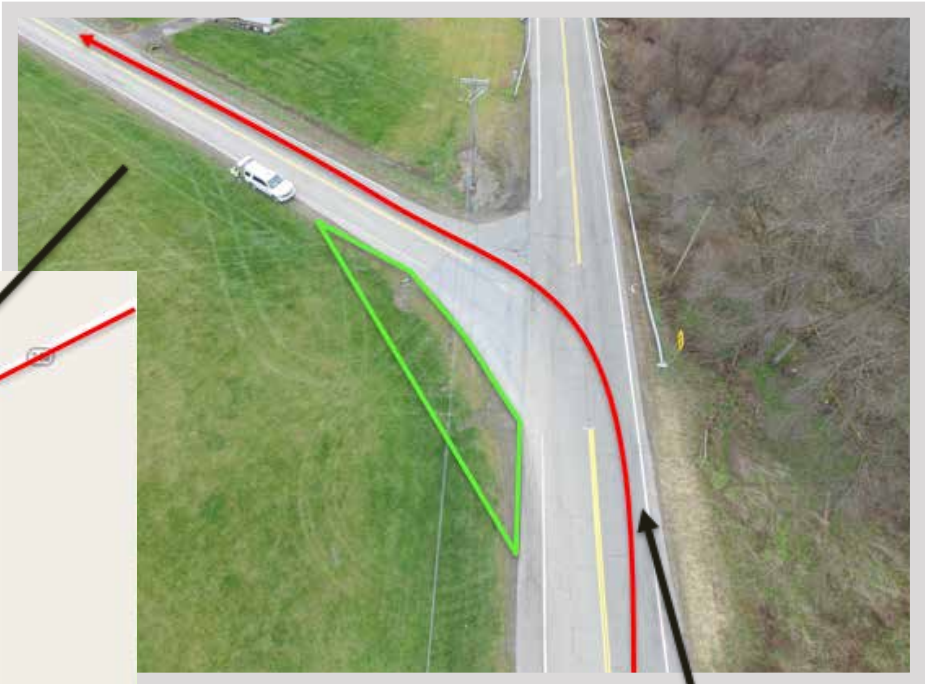
Intersection of NY248 and CR98, measured 120ft – southeast corner needs to be modified with signage removed
