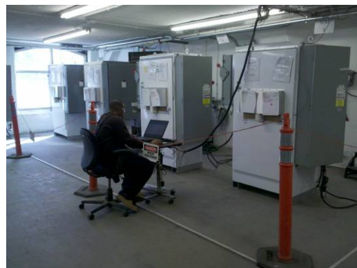
8 Hour HASS Burn-in Test and Final Verification
