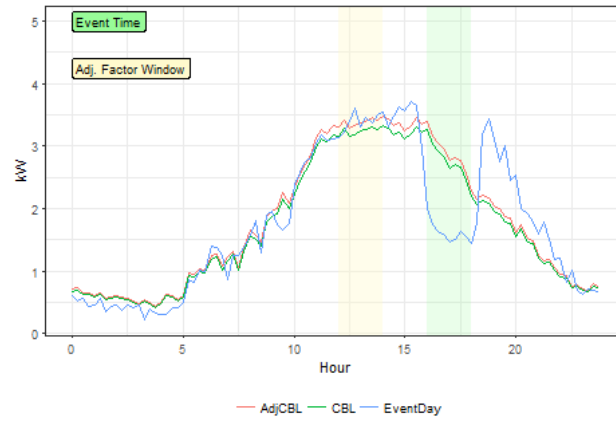
Figure 47: Small Commercial Thermostat M&amp;V Load August 16, 2018
