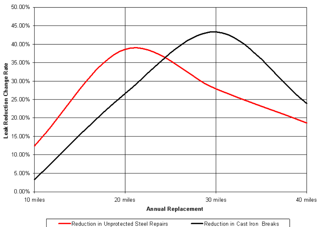
Figure 5-6: Main Replacement Impact on Leak Reduction Rates
