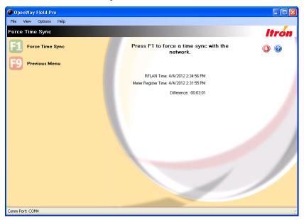
Time adjustments cause meter intervals to be shorter or longer than normal, and large time adjustments can cause whole intervals to be skipped. The meter logs a Time Change event (if configured to do so) in the meter history log, which can be seen in the Field-Pro Events window.
