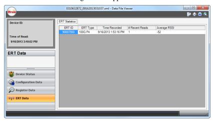
This window displays the transmission data of all ERT transmissions the meter received in the 24 hours before the data file was created. It does not display the consumption data contained in the transmissions.
