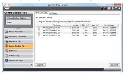
The **RF Mesh File Directory** is a fixed location to hold all RF Mesh Config files. Click **Import** to navigate and move the files to this location.
