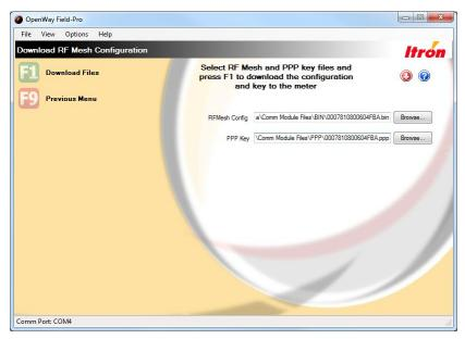
The **RF Mesh Config** file is downloaded through the register to the comm module. It contains the security certificate that authenticates communication onto the IP network, giving the meter permission to talk to the OpenWay Collection Engine.
