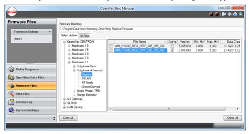
The **Select Active** tab displays all OpenWay hardware supported by OpenWay Tools. Open the nodes to drill down to the particular device for which you need firmware. When you highlight it, the window displays all firmware files located in the folder shown in the **Firmware Directory** field that can be loaded to the selected hardware. Click the **Active** check box to make the firmware file visible to Field-Pro users.
