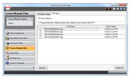
PPP Key files tell the meter's register what key to use to encrypt and decrypt information exchanged between the comm module and the register.
