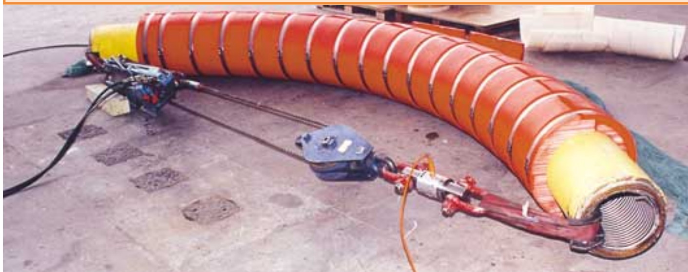
Uraduct® bend test on a flexible flowline.
