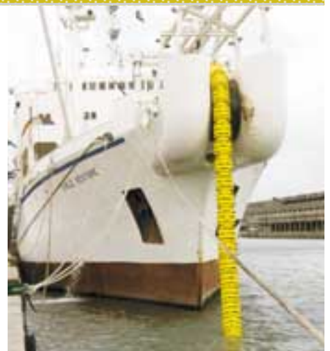
Shipboard trials for deployment and recovery of Polyspace.
