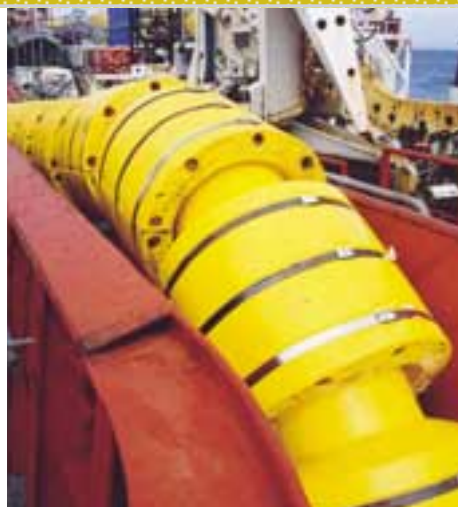
Deployment of Polyspace over cablesheet sheave.
