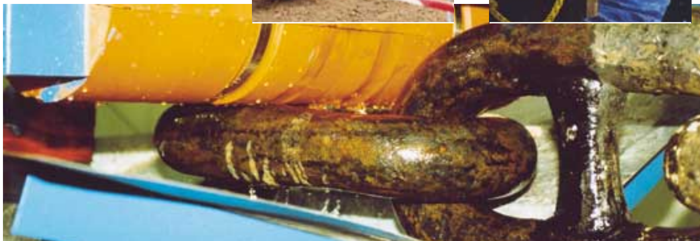
Uraduct® abrasion test against an anchor chain.
