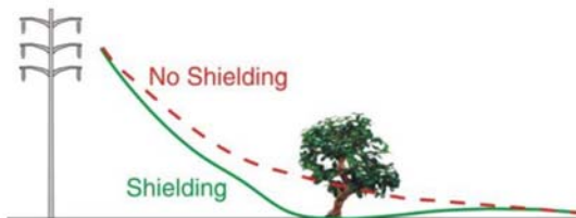
FIGURE 2-1 – ELECTRIC FIELD MEASUREMENTS DEMONSTRATE SHIELDING DUE TO THE PRESENCE OF A TREE
